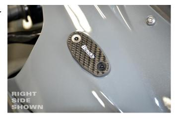
**Note**: The Nylon Washers go between the body plastic and the Carbon Fiber Mirror Block Off.
