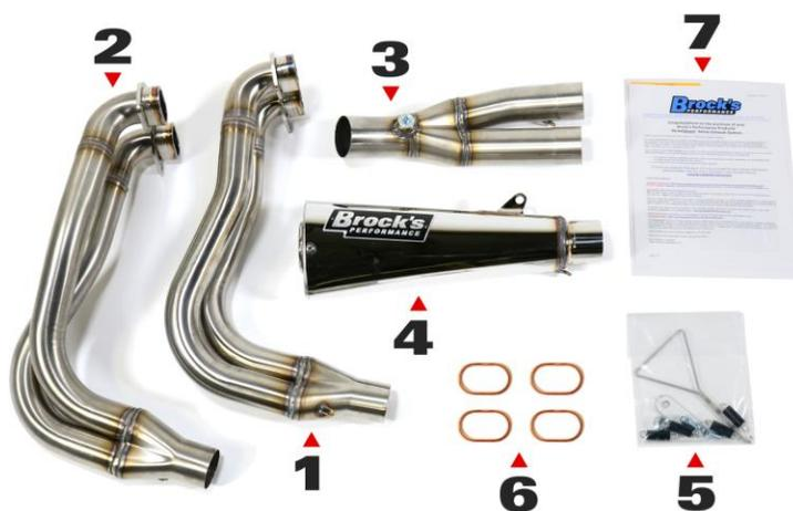
**Step 1: Pre-assemble head pipes and collector to ensure a proper fit:** Before installing the performance exhaust system, preassemble all components to check fitment. A slight ovaling of the exhaust tubing can occur during production; this is normal. Apply WD-40® to the pipe joints to ease assembly, adjustment, and disassembly (Fig 2).
