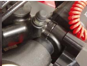
install master cylinder bracket- reassemble at dimple.
