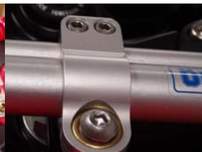
torque 8MM to: (17.2N•m/13 ft•lb) (Figure 7)
