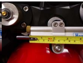
adjust position (@ 1.75 in./44.5mm) torque 5MM clamp bolts (3.4N•m/30in•lb)
