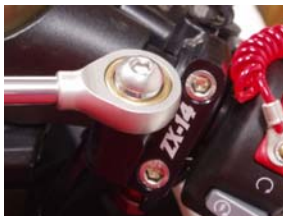
torque 8MM to: (17.2N•m/13 ft•lb) (Figure 6)
