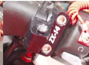
torque both screws (8.8N•m/106in•lb) (Figure 4/5)
