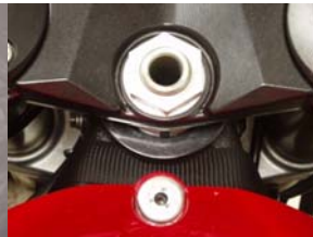
remove stock bolt -leave spacer
