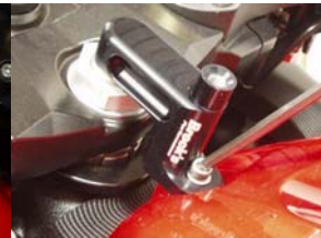
torque to: (12N•m/106in•lb) (Figure 3)
