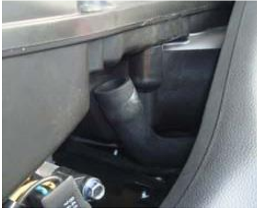
Fig. 1. AIR BOX PORT-COVER WITH BPP-S1308-CAP
