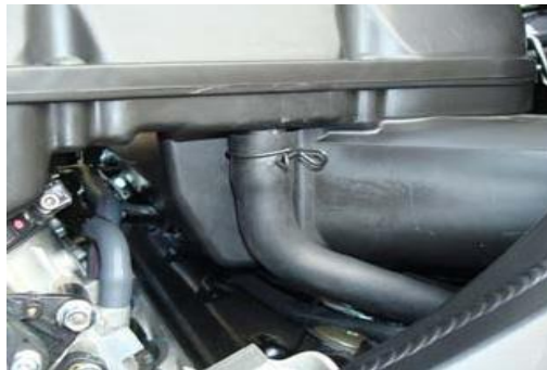
Fig. 2. REINSTALL HOSE OVER PLUGGED PORT
